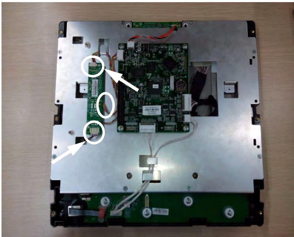
**FIGURE 3-6** Remove the inverter
