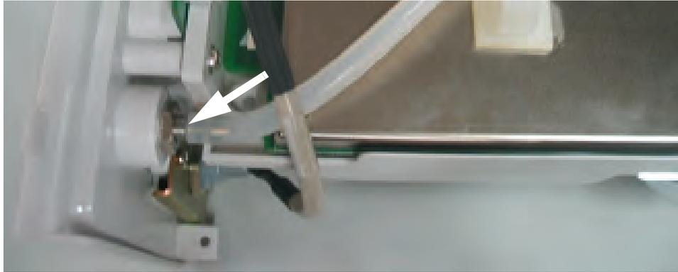
**FIGURE 3-15** Unplug the tubing from the NIBP connector
