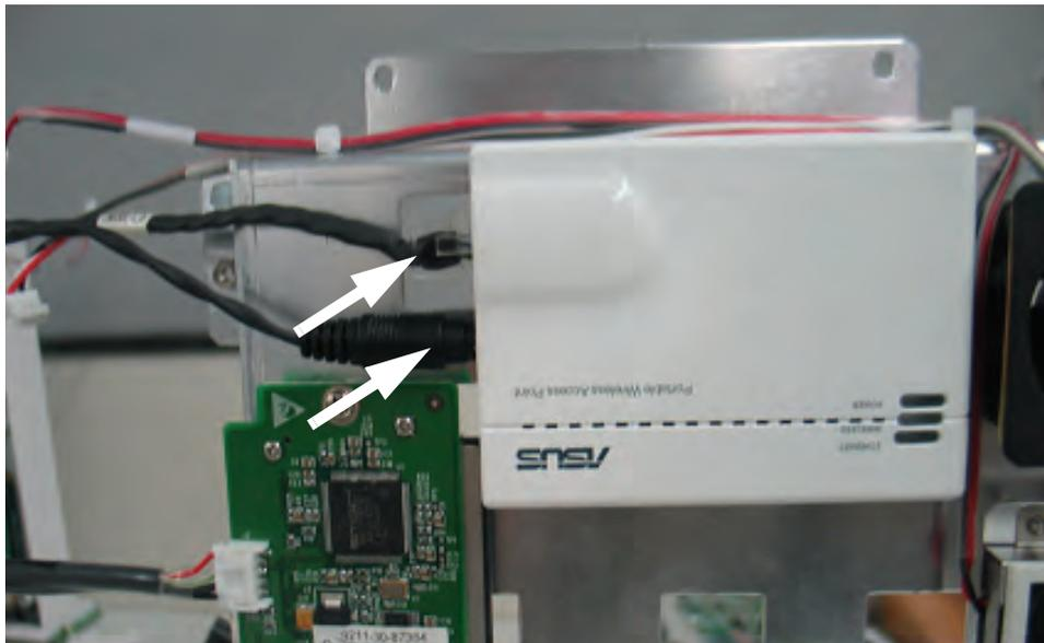
**FIGURE 3-49** Disconnect the cables from the wireless AP
