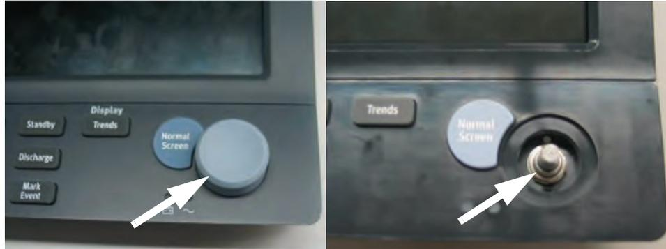
**FIGURE 3-12** Remove the encoder
