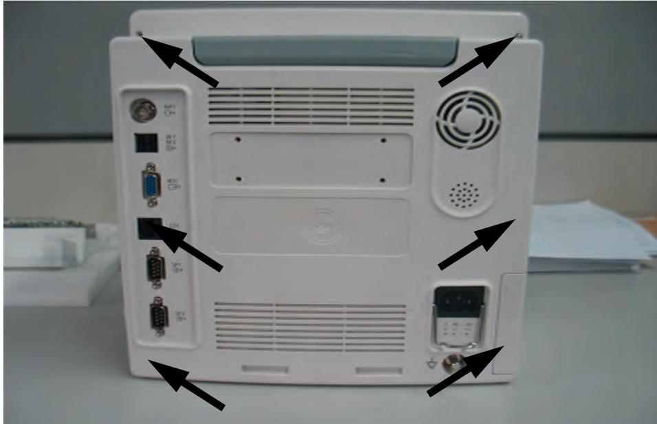
**FIGURE 3-3** Remove the screws from the rear of the unit
